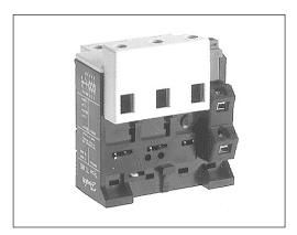
Thermal overload relays TI 80 are used with contactors CI 32-50 to give protection of squirrel-cage motors of 7.5 kW to 25 kW.
