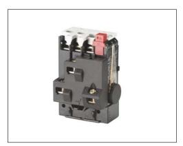
Thermal overload relay TI 9C-5 is used with minicontactor CI 5 – for protection of squirrel cage motors where compactness is required. The relay have single – phase protection, i.e. accelerated release if phase drop-out occurs.
